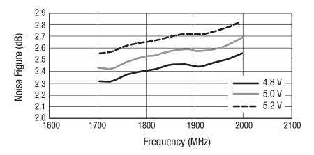
Figure 6. Noise Figure vs Frequency Over VCC
