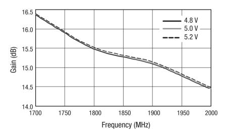
Figure 5. Gain vs Frequency Over VCC
