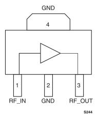
Figure 1. SKY65080-70LF Pinout – 4-Pin SOT Package (Top View)
