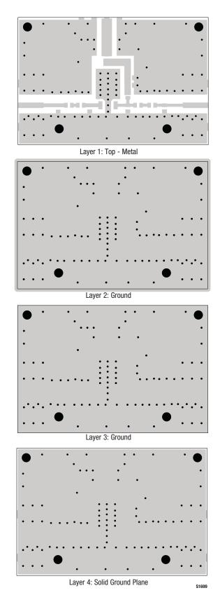
Figure 12. Evaluation Board Layer Detail
