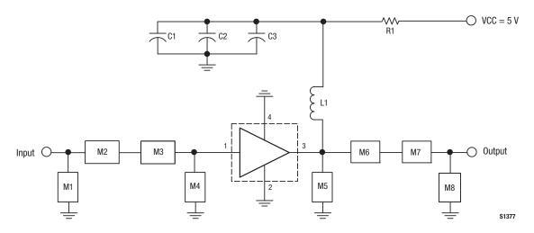
Figure 13. SKY65080-70LF Evaluation Board Schematic (1700 MHz to 2000 MHz, IIP3 Matched)
