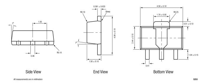
Figure 14. SKY65080-70LF (4-Pin SOT-89) Package Dimensions
