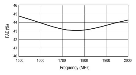
Figure 10. Power-Added Efficiency vs Frequency
