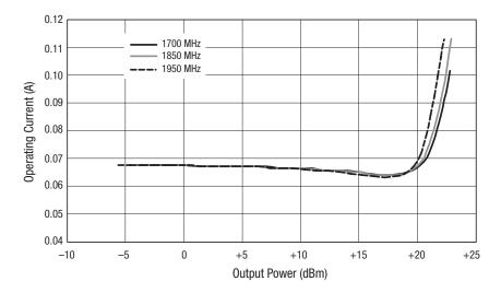
Figure 9. Operating Current vs Output Power Over Frequency
