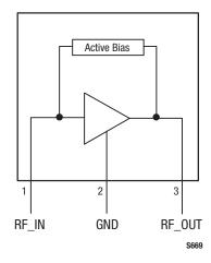
Figure 2. SKY65080-70LF Functional Block Diagram
